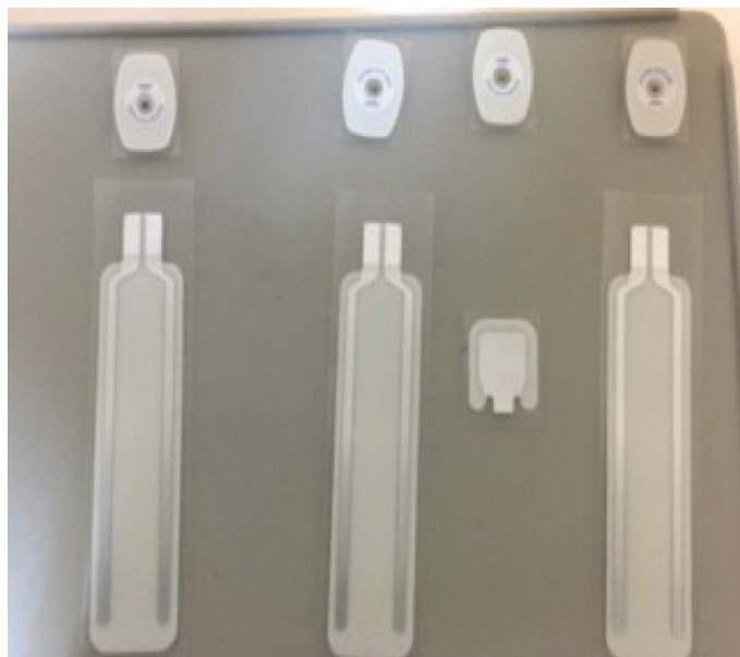
Figure 2. Electrodes used in the study (four electrodes on the upper that monitorization for patient, at lower one of them for static grounding and other three electrodes for impedance measure)
